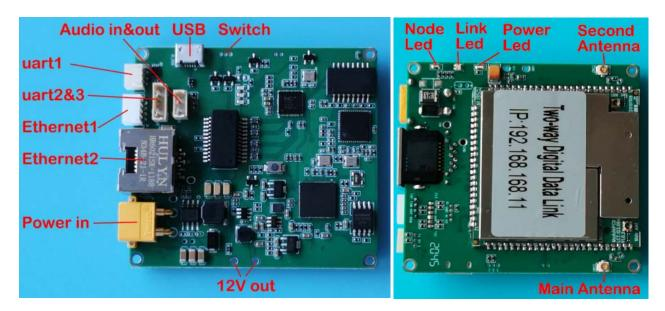
Sihid DLB module was designed for video and data wireless transmission with two way wireless data link. This OFDM radio module works at 800MHz, 1.4GHz and 2.4GHz bands, with frequency hopping technology (FHSS) to make sure better stability signal communication.
