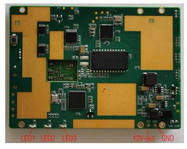
Sihid DLC module was designed for video and data wireless transmission with two way wireless data link. This OFDM radio module works at 600MHz and 1.4GHz bands, with frequency hopping technology (FHSS) to make sure better stability signal communication.
