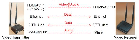
Sihid HD51 series wireless digital video transceivers was designed to capture real-time HD video with two way wireless data link. These transceivers feature HD or SD video input/output with two way OFDM modulation technology and H.265/H.264 codec that complete video audio transmission in high-speed motion with low latency. This OFDM radio works at 800MHz, 1.4GHz and 2.4GHz bands, with frequency hopping technology (FHSS) to make sure better stability signal communication.
