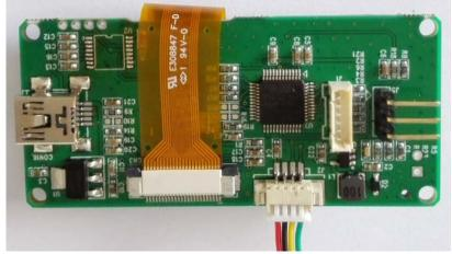
The SconC config panel has a 1.54-inch OLED display, with 3 operation buttons. SconC config panel dimensions: 65\*31mm, it does not include the connecters out of the board edge. For different Sihid COFDM modules and device case design, it should use one of the three connecting interface:
