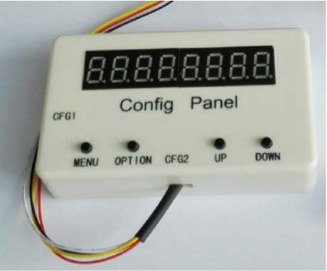
The SconB config panel has a 8 digit 8-segments LED display, with 4 operation buttons. SconB config panel is installed in a plastic outer shell, with dimensions 85\*50\*22mm. For different Sihid COFDM modules, it should use one of the two connecting interface:
