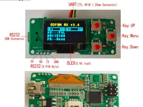
The SconA config panel has a 0.96-inch OLED display, with 3 operation buttons. SconA config panel dimensions: 54\*23.4mm, it does not include the connecters out of the board edge. For different Sihid COFDM modules and device case design, it should use one of the three connecting interface:
