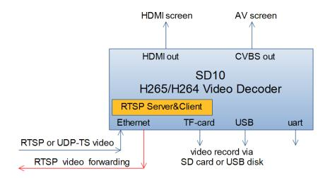
when SD10 video decoder works paired with Sihid SE11/SE10 video encoder and Sihid two-way wireless linker, the video(1080P60) latency from its inputting of SE11/SE10 to the HDMI screen displaying of SD10 is about 250ms.
