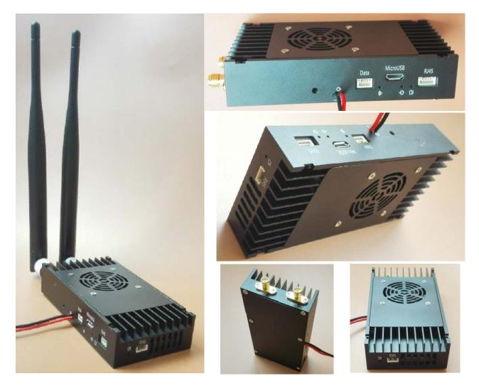
Sihid SDL530 was designed for video and data wireless transmission with two way wireless data link. This OFDM radio device works at 800MHz or 1.4GHz bands, with frequency hopping technology (FHSS) to make sure better stability signal communication.
