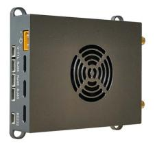
Sihid SDL600 was designed for video and data wireless transmission with two way wireless data link. This OFDM radio device works at 600MHz or 1.4GHz bands, with frequency hopping technology (FHSS) to make sure better stability signal communication.
