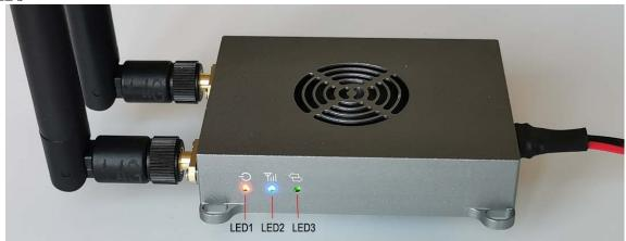
LED1, red light on normal powered; LED2, blue light LED;
