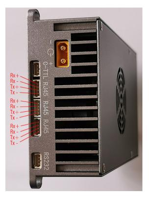
IP camera video can be connected with SDL602 directly via Ethernet port. HDMI/SDI/AHD/AV camera video can be encoded with Sihid SE10/SE11 device and then work with SDL602 via Ethernet connection.
