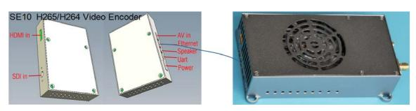
Sihid SD10 H.265/H.264 video decoder device can work with SDL602 via Ethernet connection on the video received side for realtime video monitoring.
