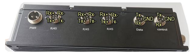
IP camera video can be connected with SDL610 directly via Ethernet port. HDMI/SDI/AHD/AV camera video can be encoded with Sihid SE10/SE11 device and then work with SDL610 via Ethernet connection.
