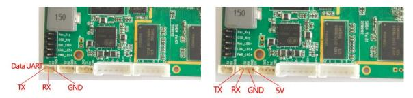
Data uart: 3PIN PH1.25mm connector, TTL 3.3V. When SHD4 board works paired with Sihid video encoder module (SUE1, SUE2, SUE3, SUE5, SUE5SA, etc.) and Ethernet linker (wireless or wire), the uart data of the encoder module will be transferred to this uart.
