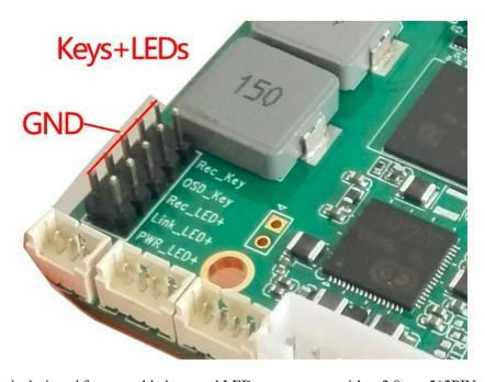
The extension port is designed for assemble keys and LEDs on necessary, it's a 2.0mm 5\*2PIN connector, please view the PCB silk printing for its' signals(as the photo above).
