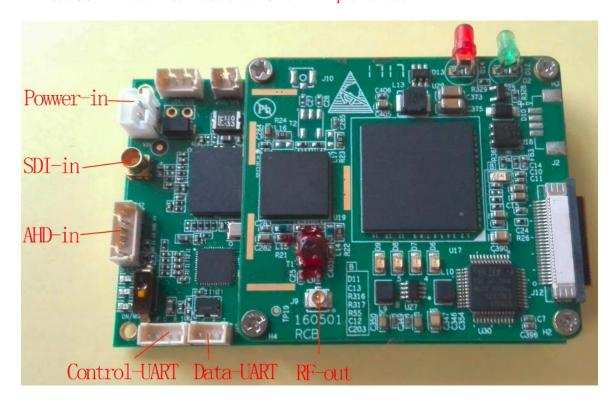
SUE5SA&RCB module features SDI/AHD(AV compatible) inputs with COFDM modulation technology and H.265/H.264 encoding that complete video audio transmission in high-speed motion and NLOS (none line of sight) conditions with low latency. SUE5SA&RCB module consists of two boards(video codec board and COFDM modulation board) with flat cable connection. The module also provides one transparent transmission uart(one way).
