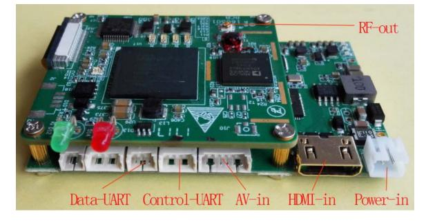
SUE5&RCB module features HDMI/AV inputs with COFDM modulation technology and H.265/H.264 encoding that complete video audio transmission in high-speed motion and NLOS (none line of sight) conditions with low latency. SUE5&RCB module consists of two boards(video codec board and COFDM modulation board) with flat cable connection. The module also provides one transparent transmission uart(one way).
