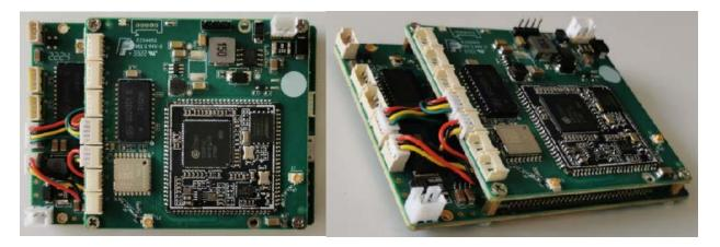
SiB1 board can be assembled with DLC wireless transceiver module with four screw holes, total weight 64.2g. The function dialog of DLC&SiB1:
